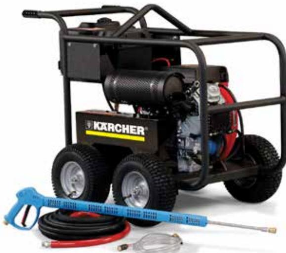
Our roll cage models are the most powerful units in our cold water line, with cleaning power of up to 5000 PSI. Protected by a rugged powder coated roll cage built of 1-1/4" steel, the PB Cage units feature powerful Vanguard, Honda or Kohler engines, tri-plunger oil bath Kärcher pumps, flat-free tires, and an extra rugged belt-drive assembly with notched V belts and cast iron pulleys. All single and double-axle models are ETL safety certified.
